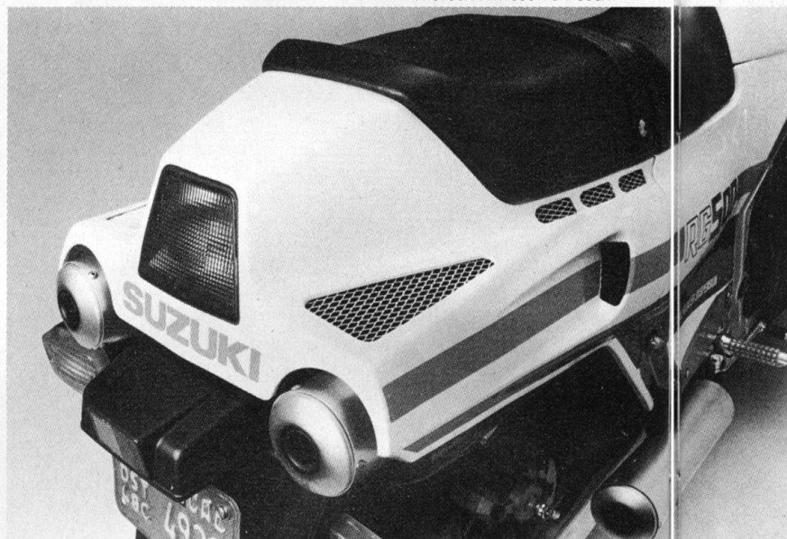
(Above) Instrument faces are classic black-on-white; bars non-adjustable. (Right) Rear pipes exit under rider; air slots help cool plumbing.
