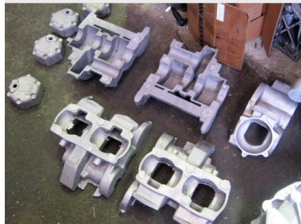
Cast engine casings ready for machining
